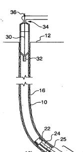
(57) Abstract: A method for drilling boreholes using casing (16) as the drill string and for advancing a casing string toward the bottom of the borehole is described. In the method, the drilling assembly (26) is used as a guide over which the drill string (16) is advanced toward the bottom of the borehole prior to removing the drilling assembly from the wellbore.
